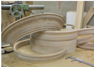
Curved oak crowns, chair rails and base boards for wrapping of large oak columns
